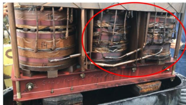
Figure-4: HT Side Short-circuited Windings
