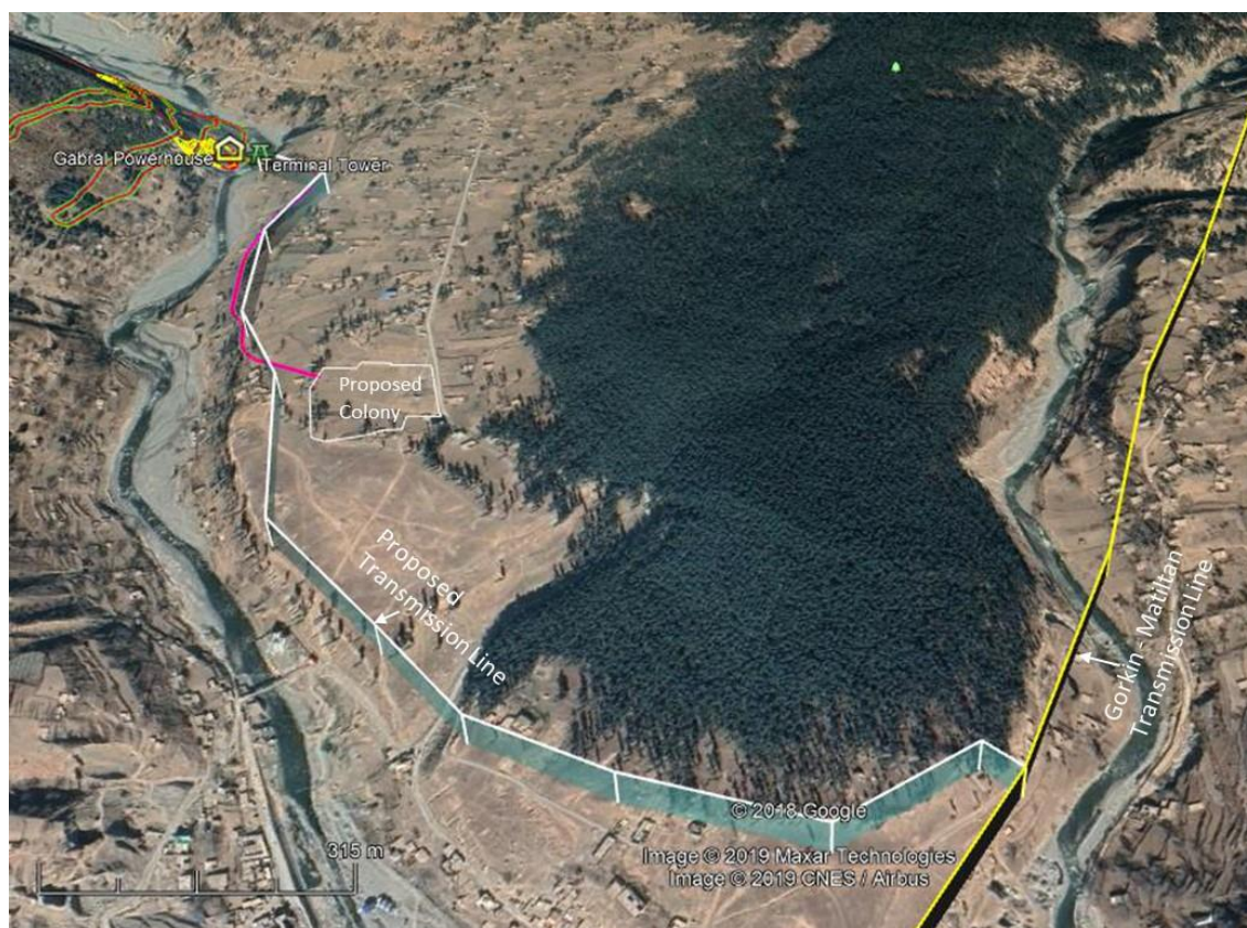
Figure 3.6: Proposed Alignment of the Transmission Line
