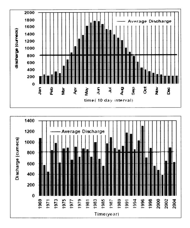
For flood frequency analysis at the Project site, the generated instantaneous flood peak data of Karot gauging station was used with observed frequency by Weibull. The highest instantaneous peak occurred in 1992. From the statistical analysis it was found that this flood caused a higher outlier in the data and hence it was truncated by trial and error
